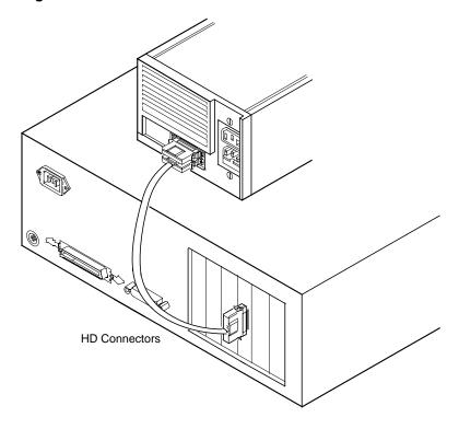
Step 3. To connect more than one external SCSI device to the host adapter, you must chain them together with shielded external SCSI cables. An example of these chained connections is shown in Figure 2.11.
